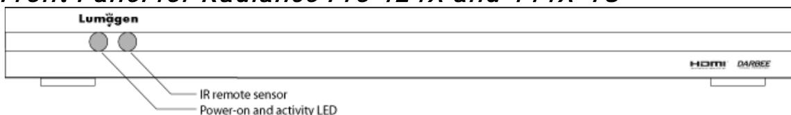
The front panel has a light-emitting-diode (LED) indicator, which is red when the unit is in “standby” and, by default, is blue when the unit is “on.” Note: The blue “on” indicator can be disabled if preferred.
